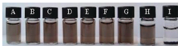
Fig. 1 Dispersions of MWNT-1 in different solutions after settling for 1 week. A: MWNT-1 after dialysis; B: MWNT-1 in 1 M NaOH; C: MWNT-1 in 0.1 M NaOH; D: MWNT-1 in 0.5 M NaCl; E: MWNT-1 in 0.1 M HCl; F: MWNT-1 in 1 M HCl; G: MWNT-1 in physiologic buffer (PBS 10 \times ); H: oxidised MWNT-1 in 0.1 M HCl; I: oxidised MWNTs in 0.1 M HCl.
